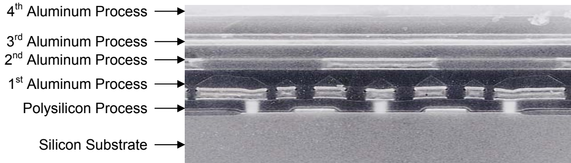
Photomicrograph of the SXR panel silicon backplane in cross section.
