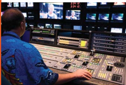
Barry Sprague at his MVS 8000G in one of NBC's master control rooms
