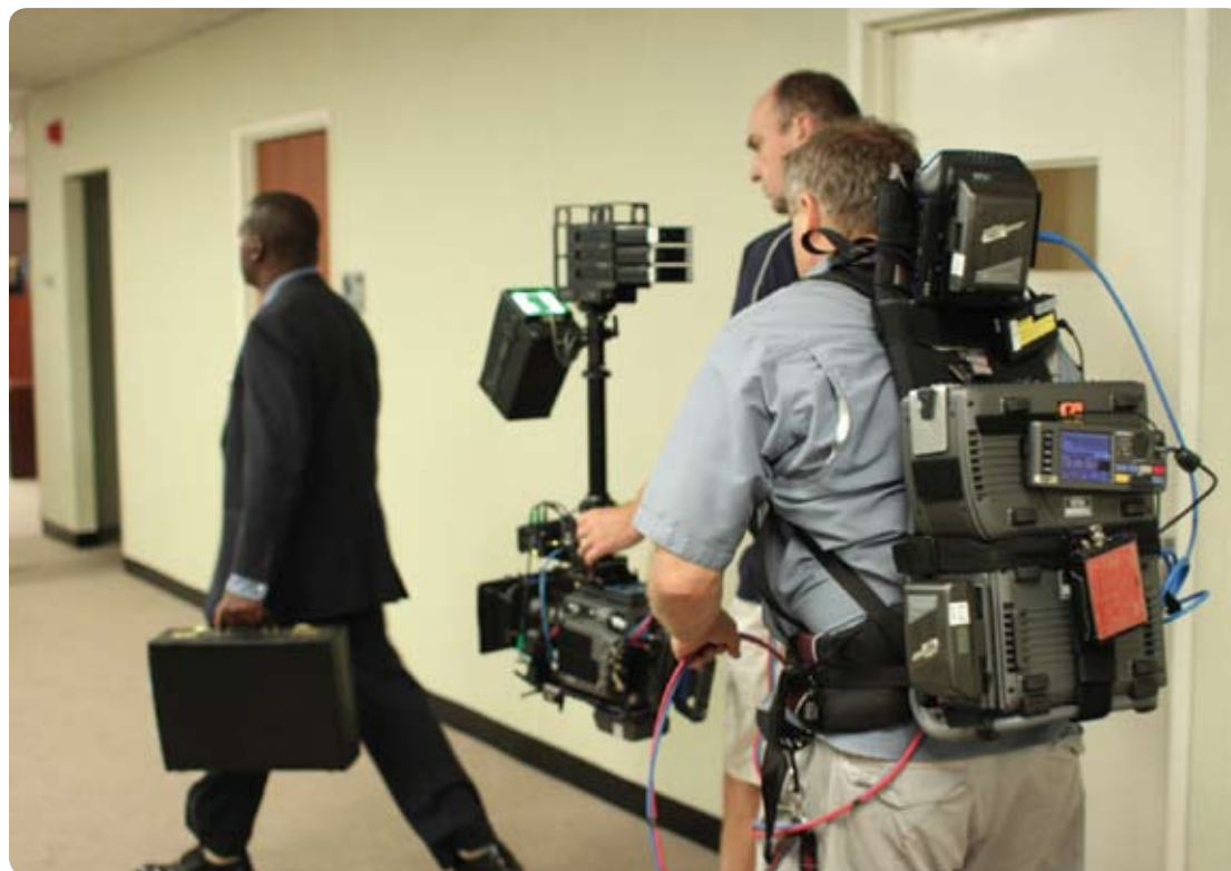
For Fox's Bones , which switched to digital acquisition this season, the production tethers the Steadicam rig to a backpack worn by an assistant. Inside the backpack is a Sony SR deck recording to HDCAM SR tape.
