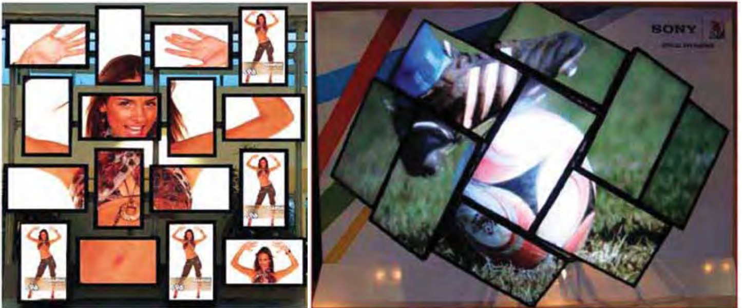
Examples of how the Sony Ziris Canvas system can be used to provide multiple images over multiple screens in an unlimited range of layouts - each screen is a large screen HDTV display
