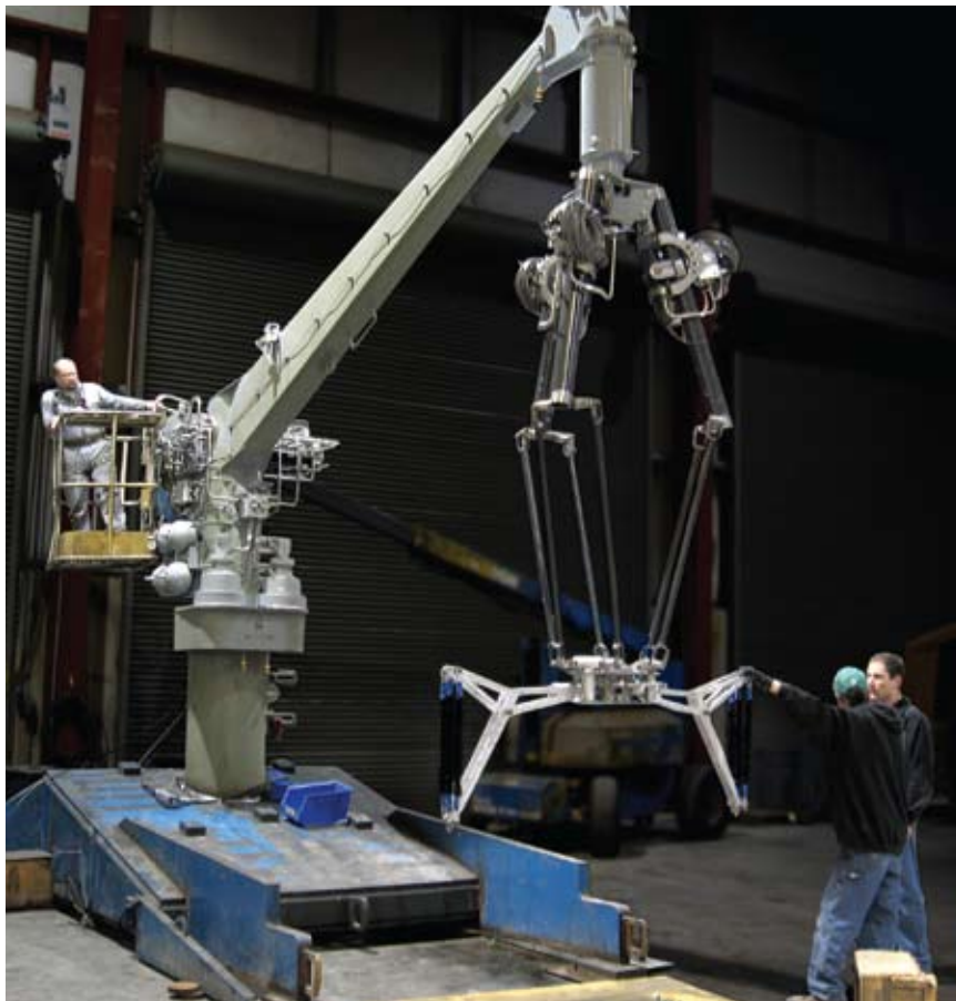
FIGURE 6. The development team constructed a fully functional scale model of the AutoLARS system. The final model will be more than 30 ft high.
