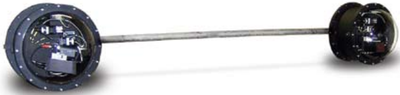
FIGURE 2. The vision system is based on two Sony XC-HR70 cameras in identical enclosures. The cameras are located about 8 ft apart.
