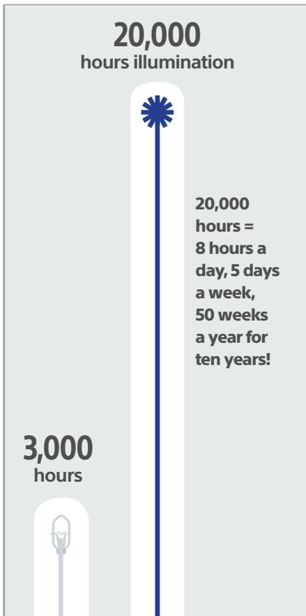
*Laser projectors have a lamp life of approximately 20,000 hours, compared to the 3,000-hour life of a conventional projection lamp.*
